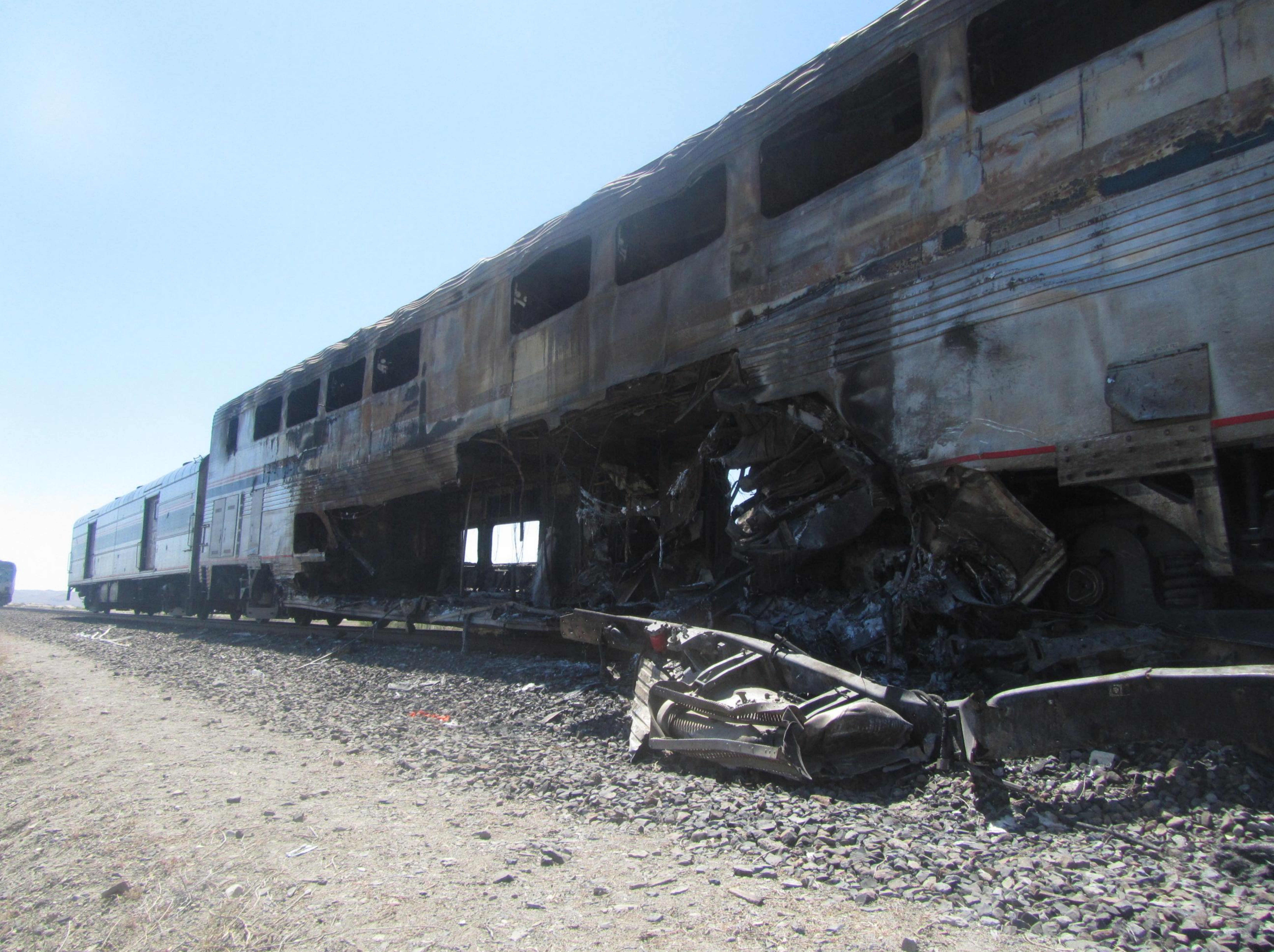
Figure 2. View of impact damage and fire damage to the Amtrak crew car.
