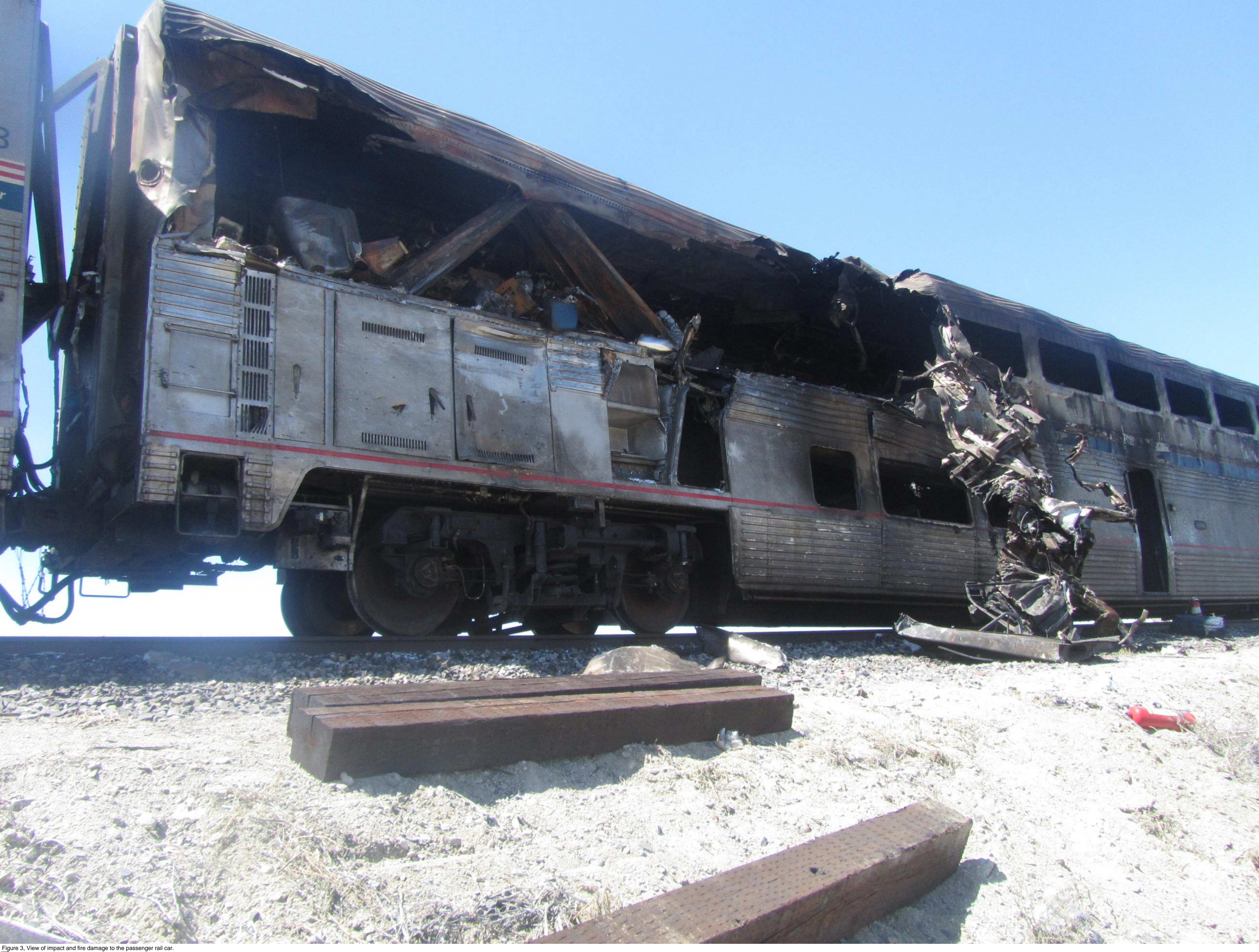
Figure 3. View of impact and fire damage to the passenger rail car.
